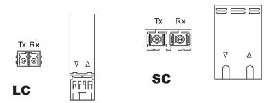
Figure 18: 100FX LC connector
